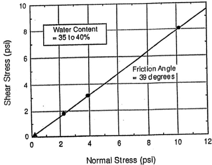
**FIGURE 3 – BENTONITE SHEAR STRENGTH AT 35 - 40% MOISTURE CONTENT**
