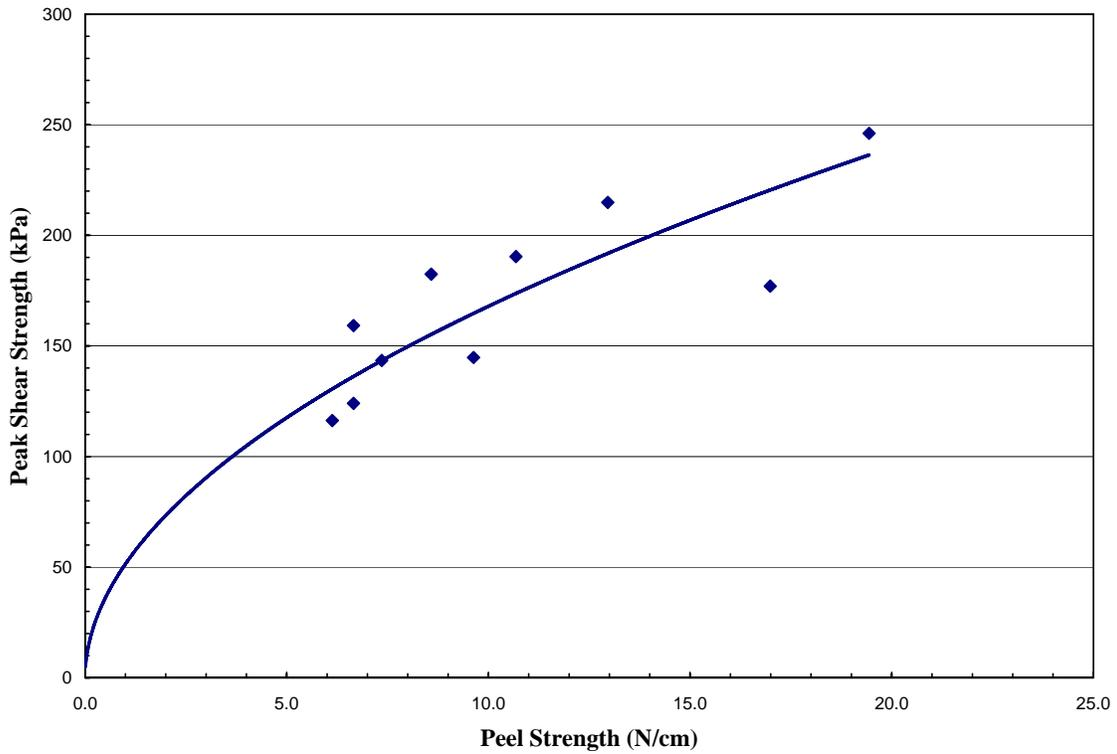
**FIGURE 2 – PEEL STRENGTH VS. GCL INTERNAL SHEAR STRENGTH**
