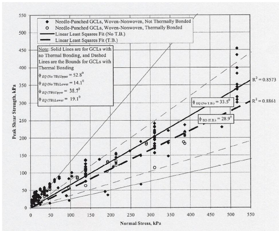
**FIGURE 4 – COMPARISON OF GCL INTERNAL SHEAR STRENGTH**
